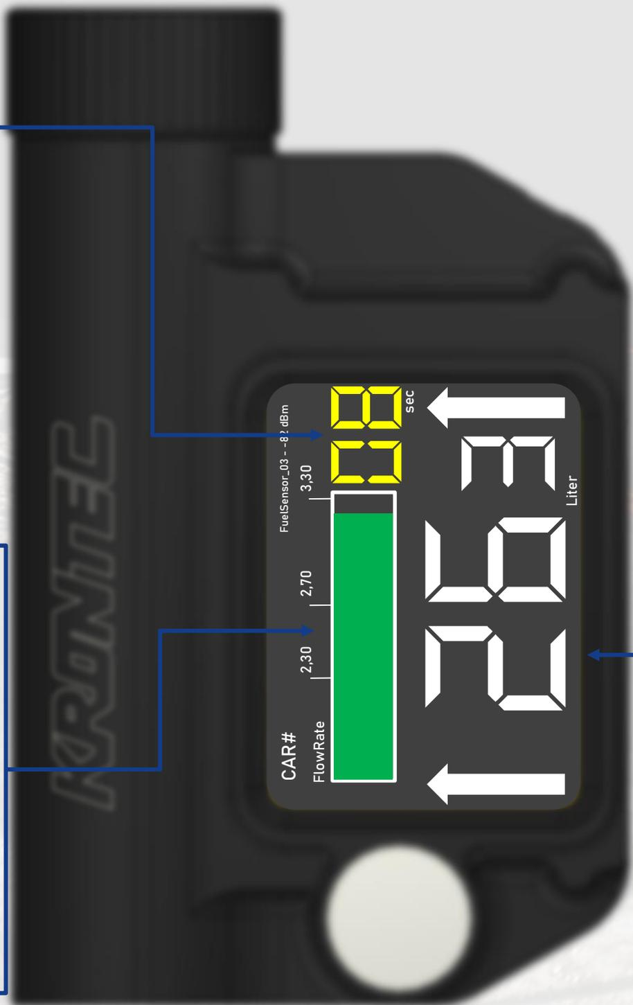
**Fuel Counter** shows the current amount of fuel depending on the mode selected. The arrows will indicate if the amount of fuel is counted upwards or backwards starting from a customizable start value.
